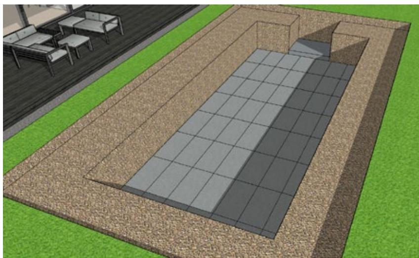
Place the XPS polystyrene on the concrete base. The polystyrene has to be under the entire surface of the pool bottom including ribs.
