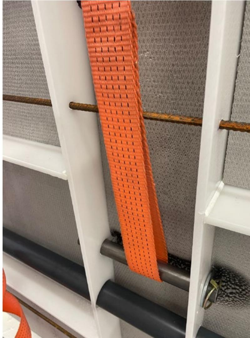
*Well placed lifting sling. Please check the lashes and washers before lifting.*
