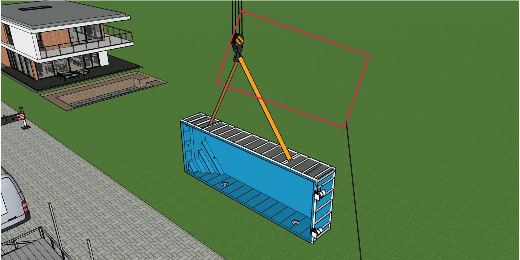
*Slowly and carefully lift the pool from the trailer - now it is necessary to move the pool to the flat place where it will be placed on the bottom and tied to 4 ties.*
