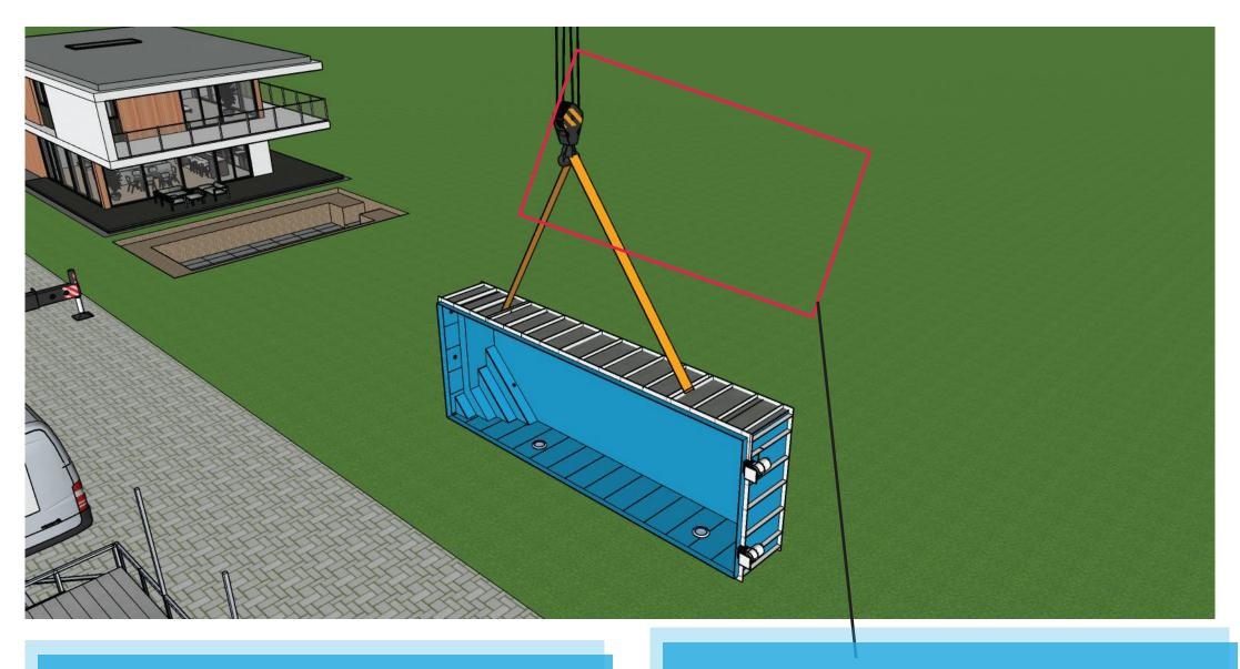
Slowly and carefully lift the pool from the trailer - now it is necessary to move the pool to the flat place place where it will be placed on the bottom and tied to 4 ties.
