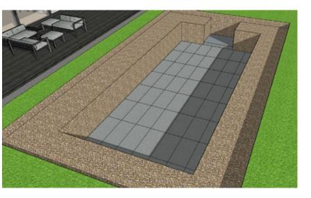
Place the XPS polystyrene on the concerete base. The polystyrene has to be under the entire urface o the pool bottom including ribs.
