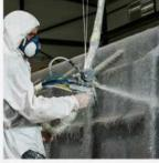
6. Fibreglass and resin spraying
