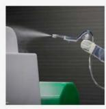
2. Application of the gelcoat, which will give the pool its colour
