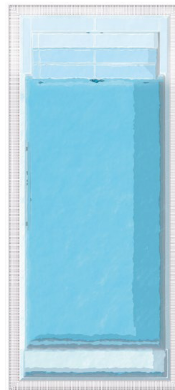
Overflow channel with stone cover adjustable overflow weir of V4A
